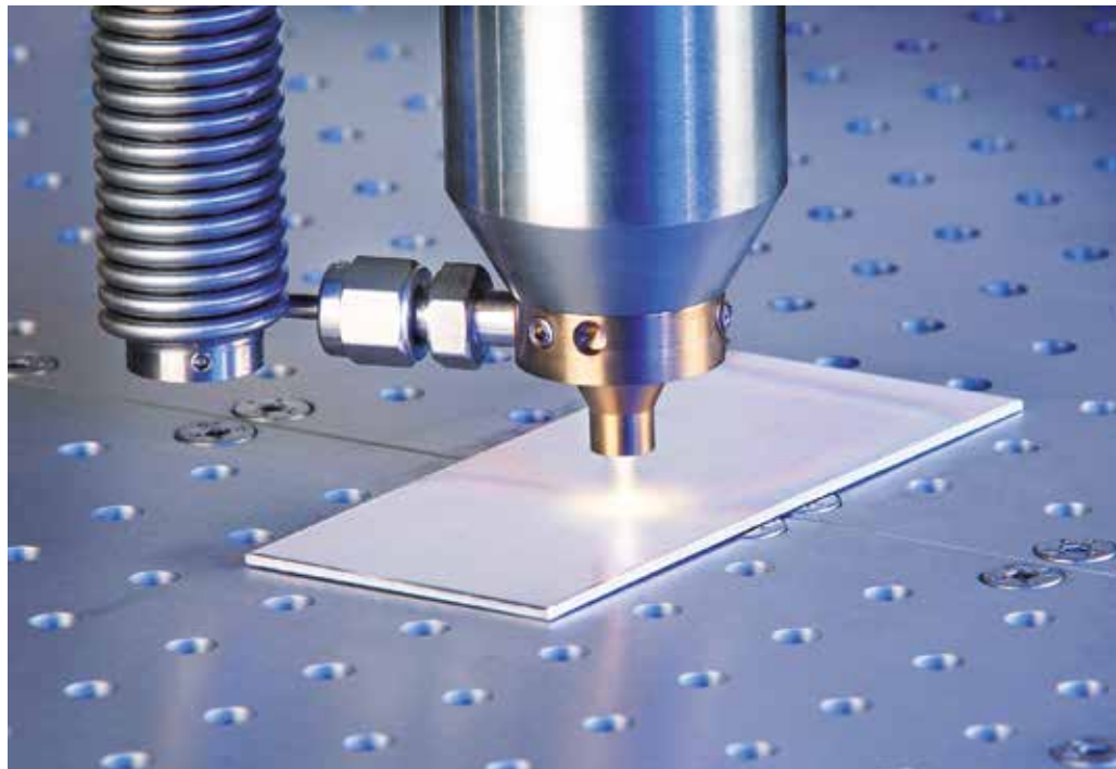
Plasma coating with atmospheric pressure: The openair plasmatechnic is operating without a vacuum chamber and due to that suitable for inline production (© Plasmatreat)
