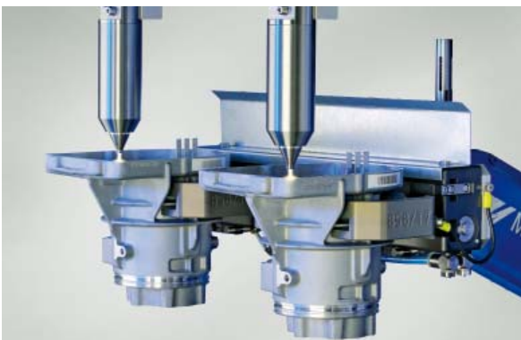
Figure 4: Prior to plasma coating TRW motor pump housings are pre-cleaned with Openair plasma to a microfine level.
