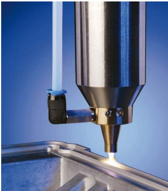
Figure 1: What was previously only achievable in the vacuum chamber is now possible in-line under normal atmospheric pressure: The functional coating of aluminium components. (Photo: Plasmamatreat)
