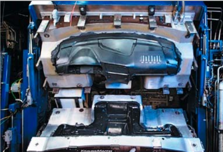
In the opened state, the foaming installation looks like a gigantic sandwich toaster. The PUR foam is applied to the black slush skin inserted below, spreads over the complete surface between the PP support structure (above) and the skin after folding up, and adhesively bonds the two parts to one another.
