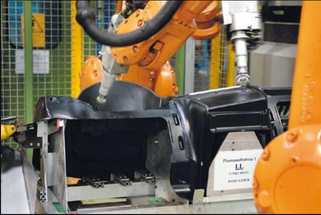
The plasma nozzles mounted to two robot arms scan the surface true to contours whilst precisely sparing those areas where no PUR foam adhesion is desired.
