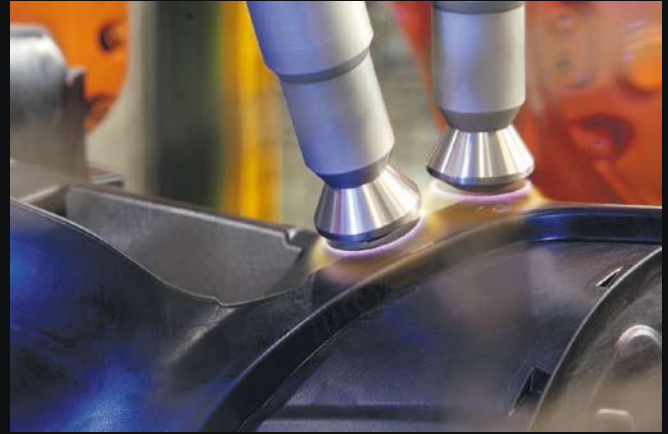
The nozzles provide selective treatment. The cold plasma brings about risk-free cleaning and activation of the long glass fiber-reinforced polypropylene surface of the dashboard even in the case of complex component geometries.
