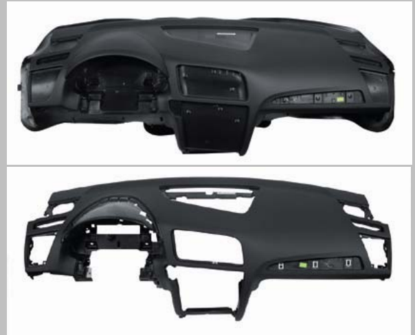
Instrument panel after plasma treatment. Adhesive slush skin and foam bonding and rear-side skin weakening in the area of the air bag (above). A milling system produces the instrument openings. The back-foamed slush skin can be easily removed by hand from the non-plasma-treated areas.
