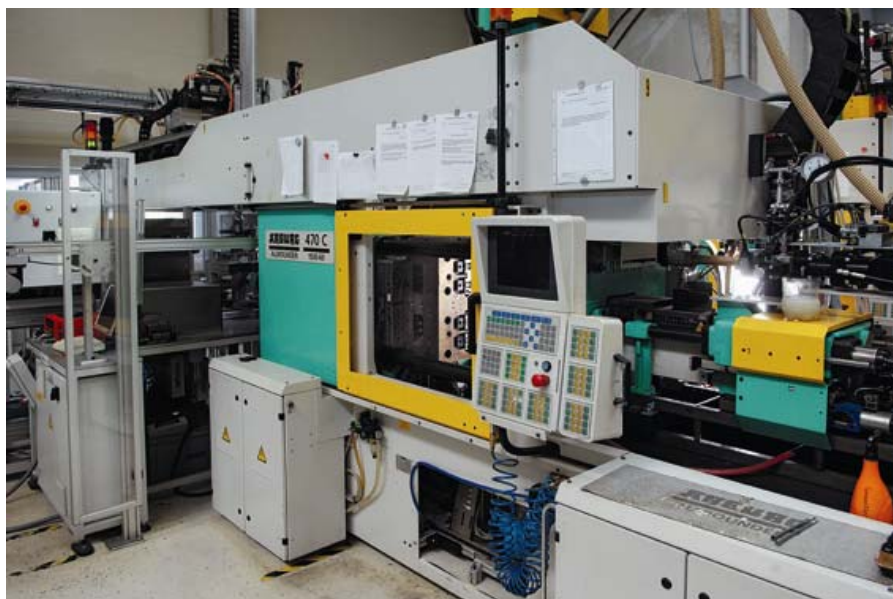
Fig. 5. Sophisticated integration solution: A pneumatic motion system moves the plasma nozzles from downwards into the injection molding section of the machine
