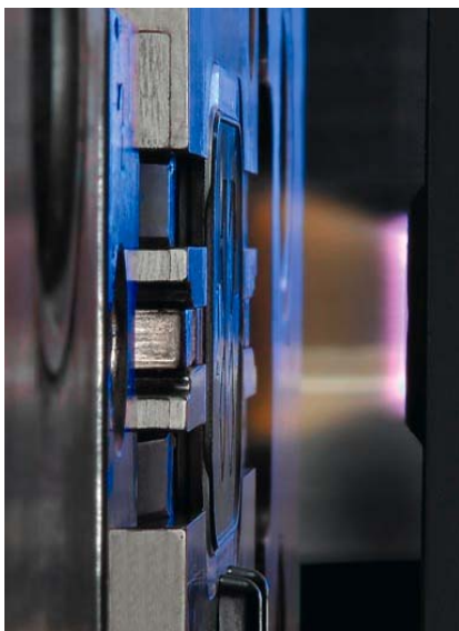
Fig. 4. View into the injection molding machine: The Openair plasma beam impinges with almost ultrasonic speed on the polycarbonate lenses. Microfine cleaning and strong activation impart new adhesion properties to the plastic material
